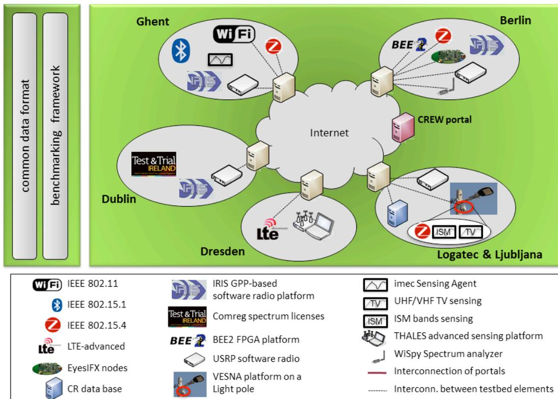
**Figure 1: The CREW federation of cognitive radio testbeds**
